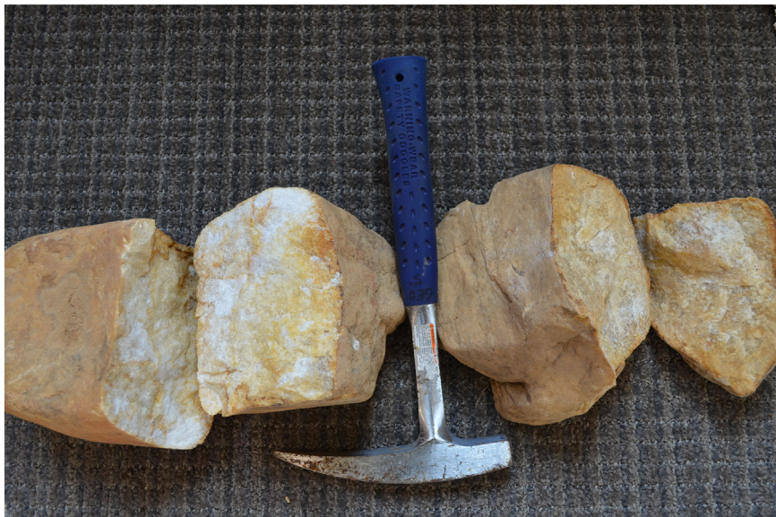
Fig. 3. Split quartzite cobbles sampled from terraces along Brushy Creek (left of hammer) and Threemile Creek (right of hammer).
