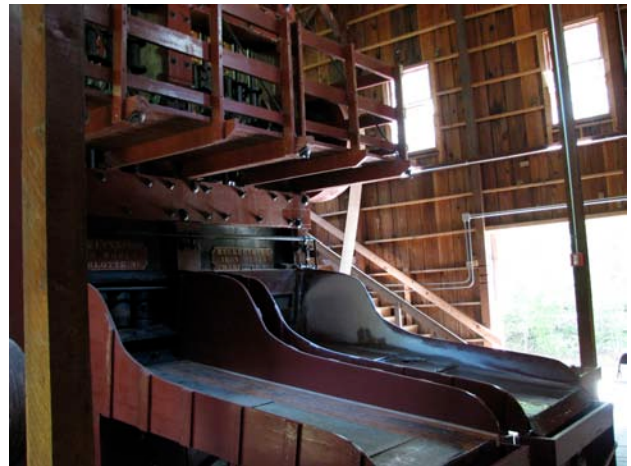
Figure 27. The stamp mill at Reed Gold Mine.
