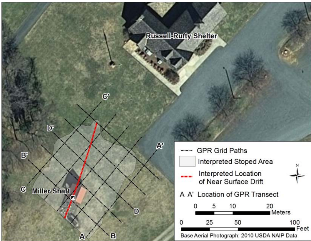
Figure 8. Map showing location of GPR transect lines and extent of stoping interpreted from GPR data. Miller shaft area - Gold Hill Historic Park, Gold Hill, NC.
