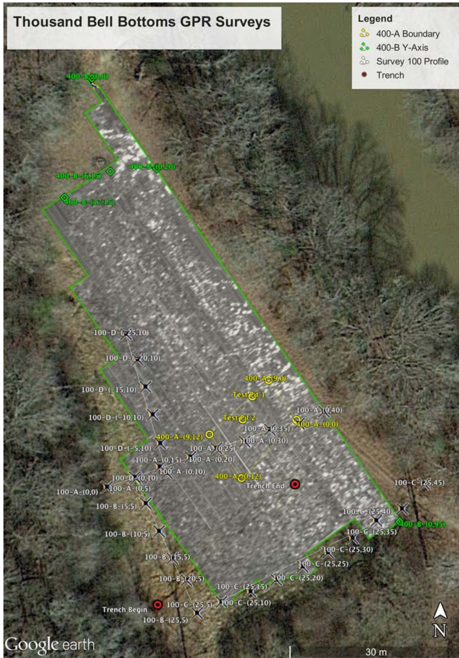
Figure 3. Thousand Bell Bottoms GPR survey locations. The Uwharrie River is to the east in the image. Survey 400-A boundaries and corner points are near the center of the image. The footprint of Survey 400-B is laid out by boundary lines, and an integrated Z map fills the footprint. The Z map shows radar features within the 2.2 m thick horizontal slice. Bright spots are stronger positive anomalies. The lines for Survey 100 sections are shown as white lines with waypoints every 5 m. Endpoints of a trench excavation are denoted with targets.
