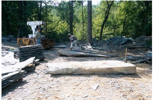
Figure 15. Splitting operation at Jacob's Creek quarry.
