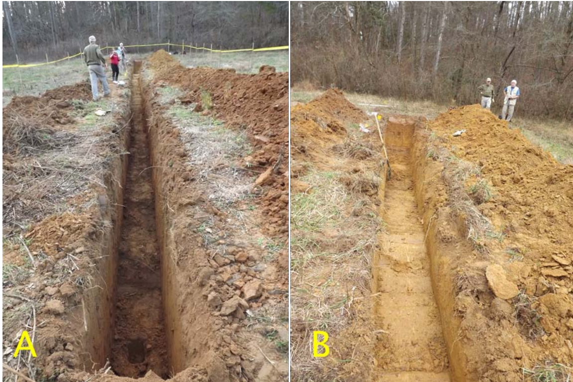
Figure 4. Completed backhoe trench at TBB. (A) The look direction is toward the southwest. Forest Road 555 is behind the trees in the distance. In the foreground, the floor of the trench is saprolite of Tillery Formation. Several round cobbles were recovered in situ from the trench floor here and mark the strath. (B) The look direction is toward the northeast. The soil/sediment is yellow-orange below a shallow brown-orange horizon that is inferred to be the near-surface, lower frequency horizon that occurs throughout TBB.
