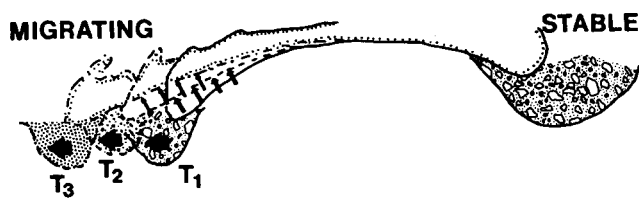
Figure 10. Trailing barrier realignment. Updrift erosion is a consequence of inlet migration and the associated planform adjustment.
