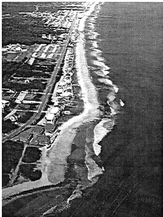
Figure 33. Fort Fisher aerial photograph. North view (1987). The beach along the Fort Fisher/Kure Beach section is perched atop Pleistocene units comprised of two lithologies: Coquina and a friable humate rich sandstone. Coquina crops out on the beach front of the townhouses in center of photo. The underlying geology plays a critical role in the local erosion.
