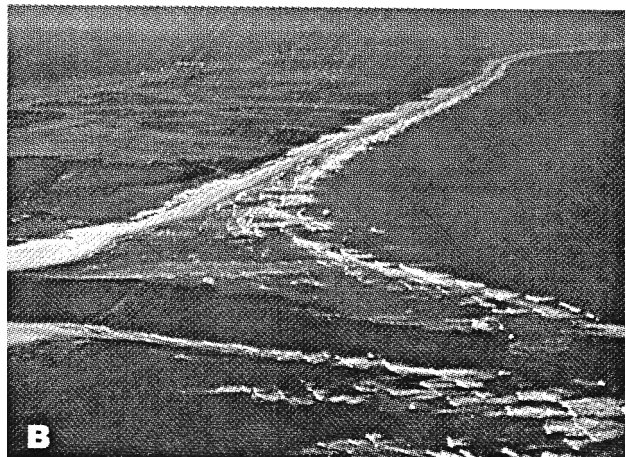
Figure 30. Masonboro Island aerial photographs. North view of Masonboro Island (1981). Storm deposits characterize the barrier. Since the 1980's the island has receded rapidly. The 1996 shoreline is located within the maritime forest in the center of the photo. North view (1994) of Masonboro Island from Carolina Beach Inlet. The southern segment of the barrier is low and eroding rapidly due to the opening of Carolina Beach Inlet in 1952. Overwash during storms is the driving variable that is most important in island migration. Currently the area shown is a single continuous washover terrace.
