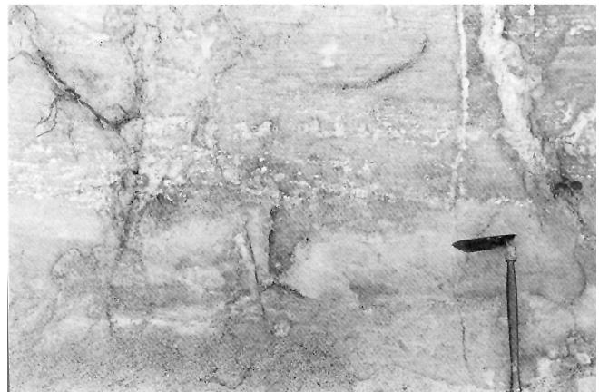
Figure 15. Typical roadcut exposure of upland unit clayey grit with clay balls and cross-beds, southeastern \frac{1}{4} Foxtown quadrangle.
