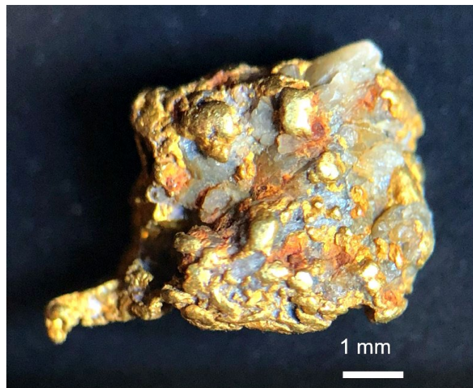
Figure 12: Gold in quartz from palladium-bearing gold prospect. Sample recovered from a depth of 100 feet within rotary drill hole. Gold stands out in relief as rounded nuggets within saccharoidal quartz.
