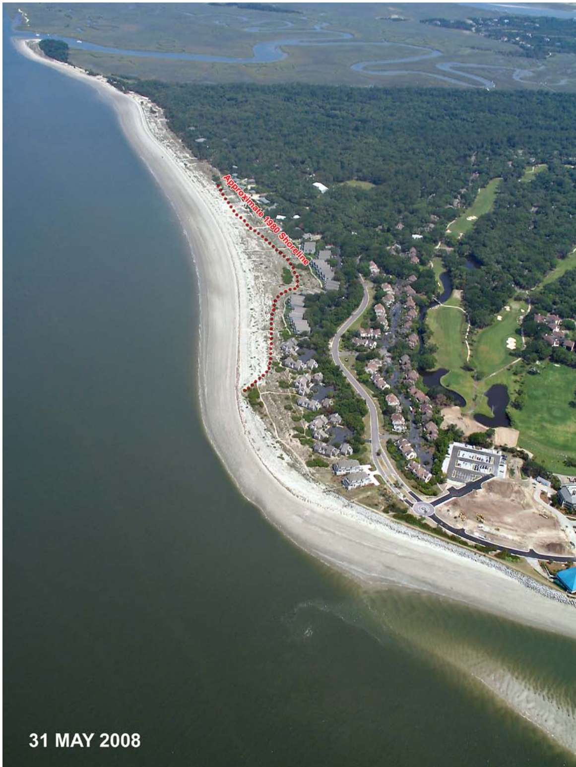
19. The Seabrook Island shoreline from Beach Club Villas (lower edge of image) to Camp St. Christopher at low tide on 31 May 2008. Peican Watch Villas were originally aligned with the shoreline when built in the 1970s. Dotted red line marks approximate shoreline in 1980. Photos by TW Kana.
