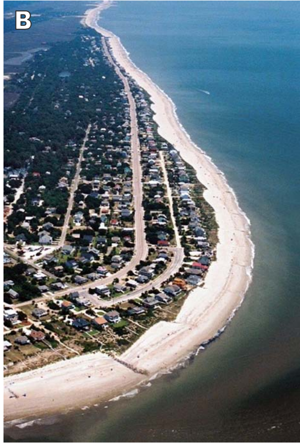
27. Aerial views of Edisto Beach taken on 10 February 2006 (A) before a major beach nourishment project and after it in June 2006 (B). Note how the nourished sand had buried many of the groins. Photographs by Tim Kana.
