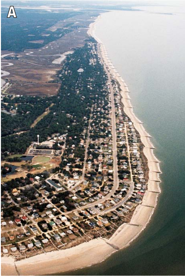
27. Aerial views of Edisto Beach taken on 10 February 2006 (A) before a major beach nourishment project and after it in June 2006 (B). Note how the nourished sand had buried many of the groins. Photographs by Tim Kana.
