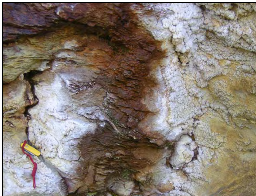
Figure 5. White gypsum blooms, yellow (jarosite?), and dark orange oxide coatings on sulfidic metagraywacke exposed adjacent the June 15, 1999 rockslide (CER-001) near Crabtree Meadows. The NNP test value for this rock was -22.02 as shown on Figure 4.
